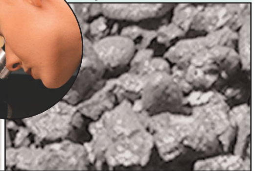
GreensandPlus magnification: 50X
